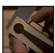
If the square is too obtuse (greater than 90 degrees), loosen the acute adjuster screw slightly and tighten the obtuse adjuster screw until snug. Repeat until square.
