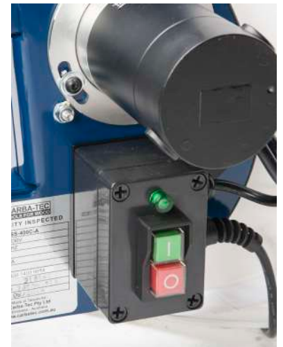
NVR power isolating switch
